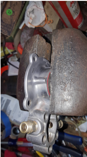
FIGURE 12 Gently apply pressure to Outer Seal until it is flush with face of Bearing Cap.
