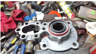
FIGURE 3 Bearing Cap with first of two new seals in place, waiting to be installed.
