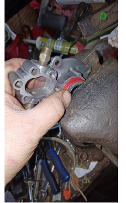
FIGURE 11 Carefully align Outer Seal in hole in Bearing Cap before applying pressure with vise.
