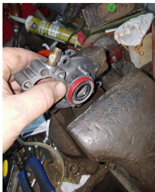
FIGURE 4 Place Bearing Cap and Seal in vise.
