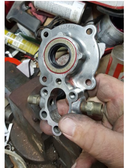
FIGURE 13 New seals installed.
