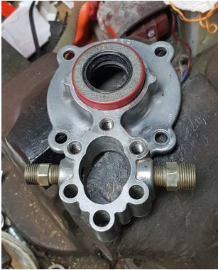
FIGURE 10 Correct placement of Outer Seal.
