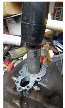
FIGURE 2 Removing old seal from Bearing Cap.
