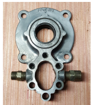
FIGURE 1 Bearing Cap with original seal installed.
