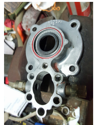
FIGURE 7 First (inside) Seal installed.
