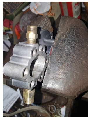
FIGURE 6 Seal pressed in all the way.
